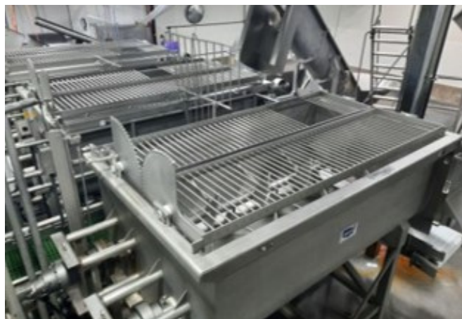
AMFEC approximately 8,000 LB Capacity Stainless Steel Dual Shaft Paddle Blender
